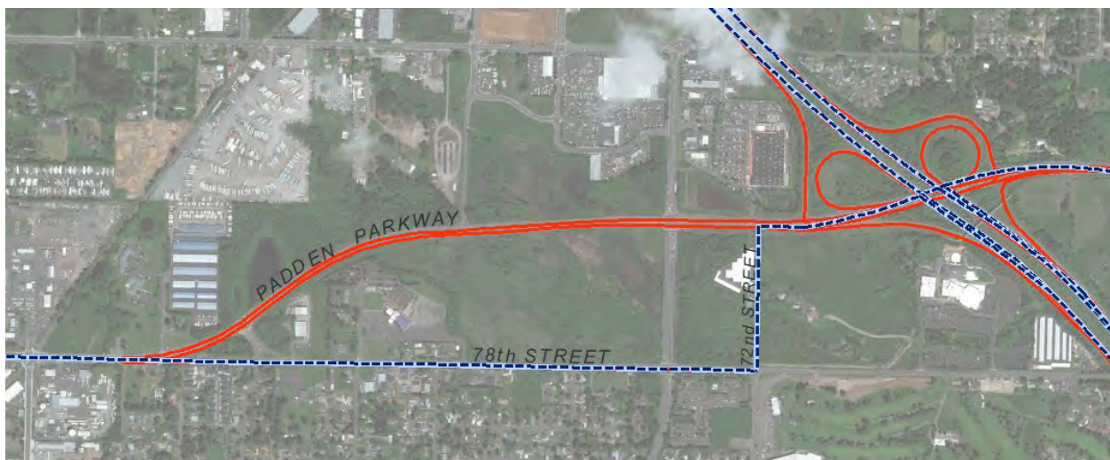
Figure 5. Road improvements and approaches were incorporated. For example, 72 nd Street no longer connects 78 th Street and what was 83 rd Street. 83 rd Street has been replaced by Padden Parkway. In addition, the old ETRs (in blue) did not include highway ramps.
