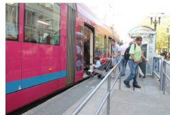
Level boarding platforms for bus, streetcar and MAX improves service for passengers and reduces loading and unloading times.
