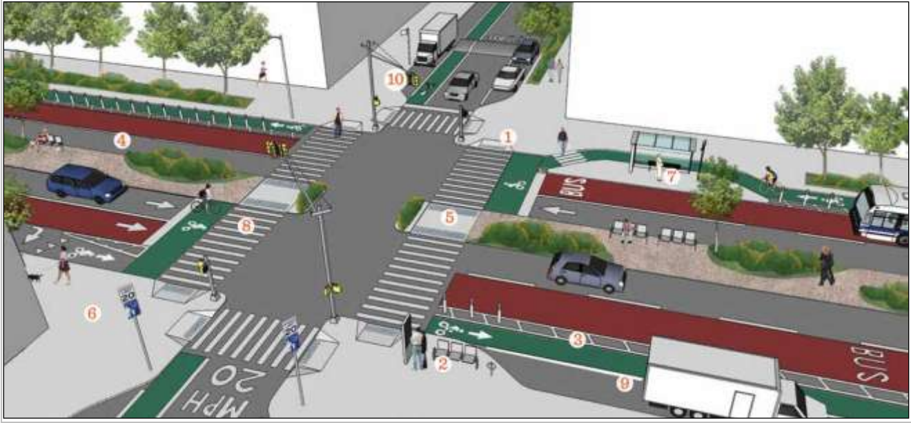
Figure 45: Example of a vision zero street (1)ADA accessibility, (2)public amenities, (3) protected bike lanes, (4) narrow vehicle lanes, (5) pedestrian islands, (6) wide sidewalks, (7) dedicated mass transit facilities, (8) signal protected pedestrian crossings, (9) dedicated unloading zone, (10) signal retiming
