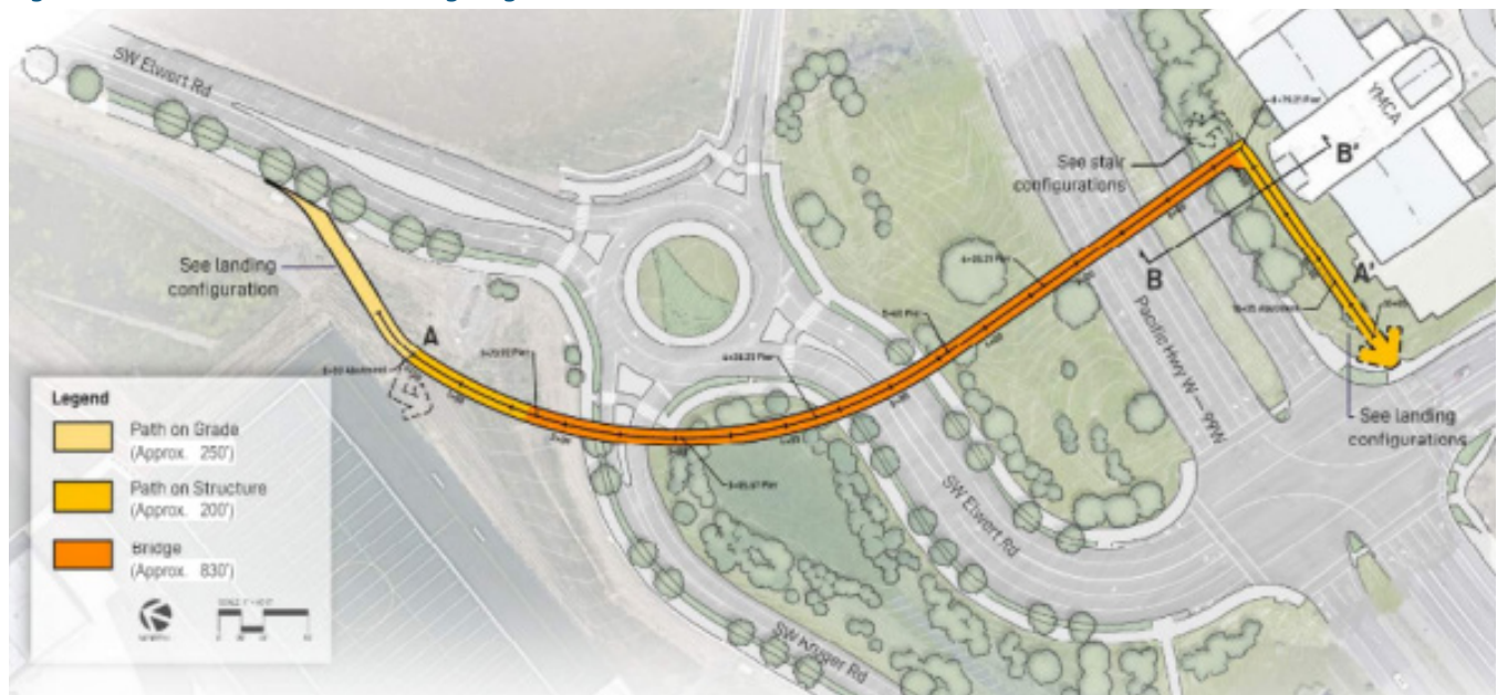
Figure 18. Pedestrian Overcrossing Alignment
