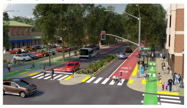
Rendering of a Regional Street showing a four-lane street with a planted median, crosswalks, and buildings. One lane in each direction is a bus only lane. There is a bus and four cars. A painted green bikeway and sidewalk are separated from the roadway by a planted median. People are walking and crossing the street. Source: Metro Designing Livable Streets and Trails Guide
