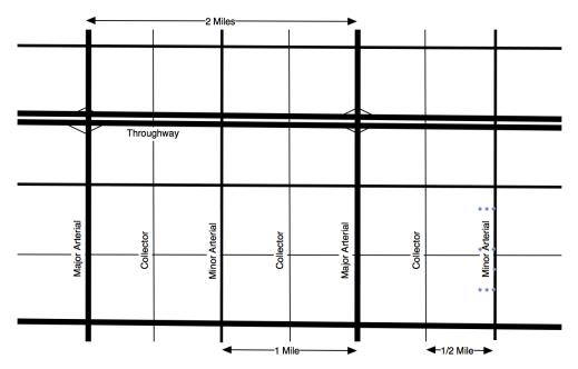
Figure 3-21 Regional motor vehicle network concept
