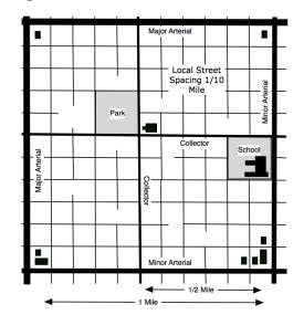
Figure 3-22 Collector and local street network concept
