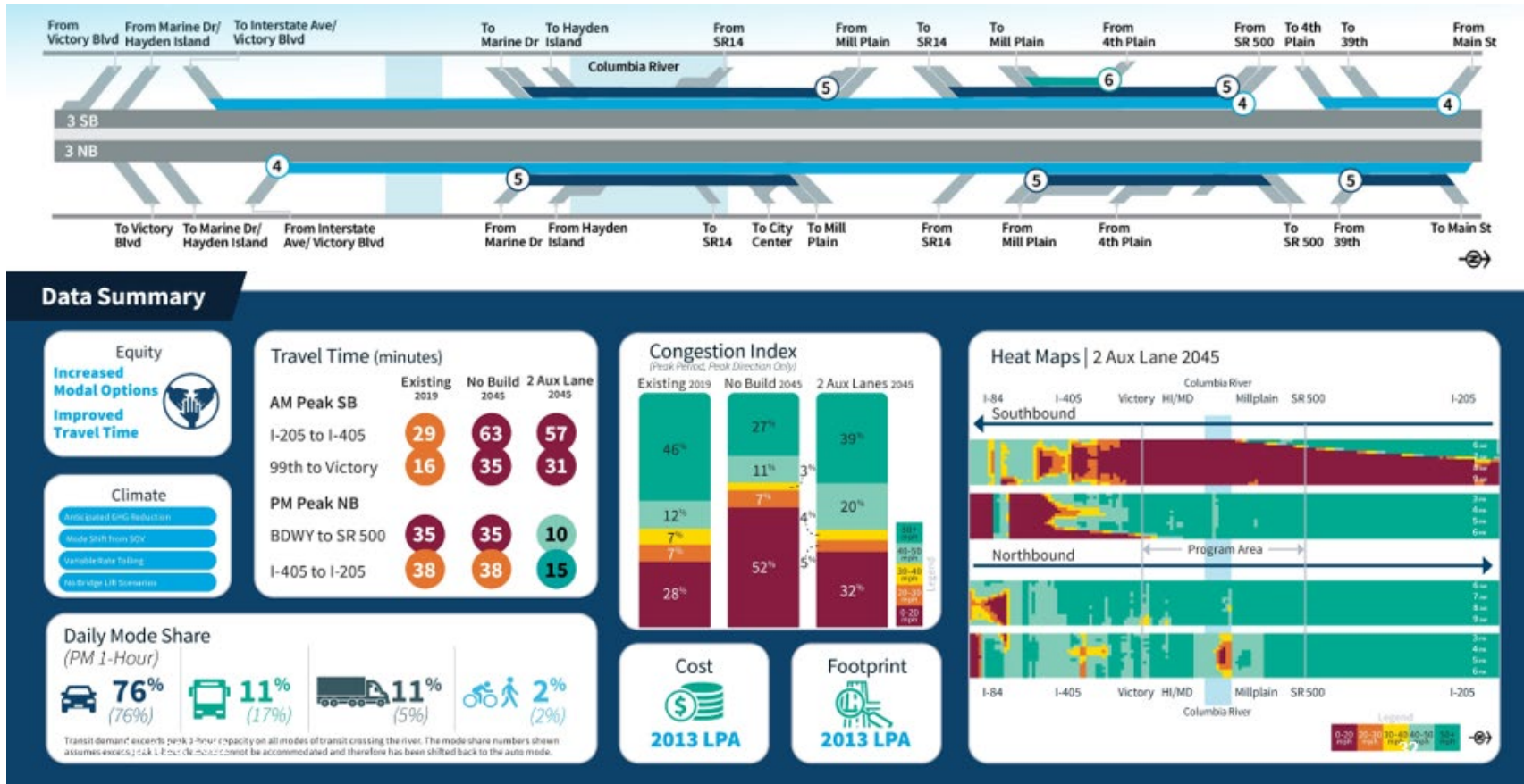
Figure 19. Auxiliary Lanes – Two Auxiliary Lanes
