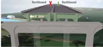
1. Construct new bridge foundations, widen each side. Slide one direction. Existing lanes will remain open to traffic during this time. (Phase 1A)
