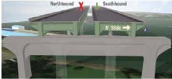
2. Slide the other direction. Existing lanes will remain open to traffic during this time. (Phase 1A)
